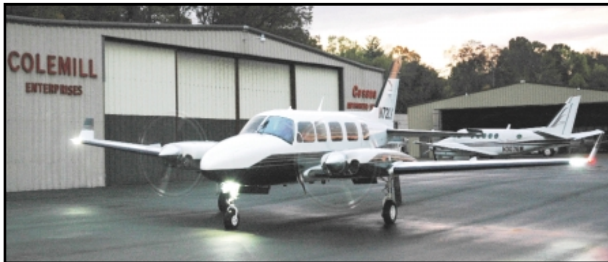
Colemill now offers its popular Panther modifications with either standard rotating or counter rotating engines.
