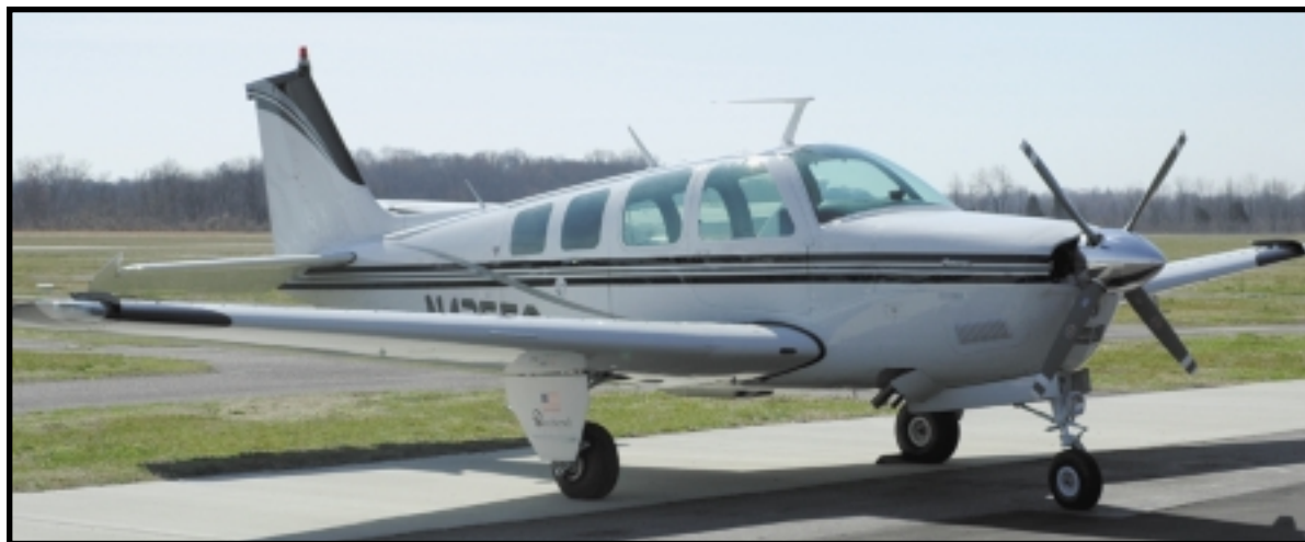
Chip Johnson says the Starfire's four blade “Q-Tip” propeller makes his Bonanza much smoother.
