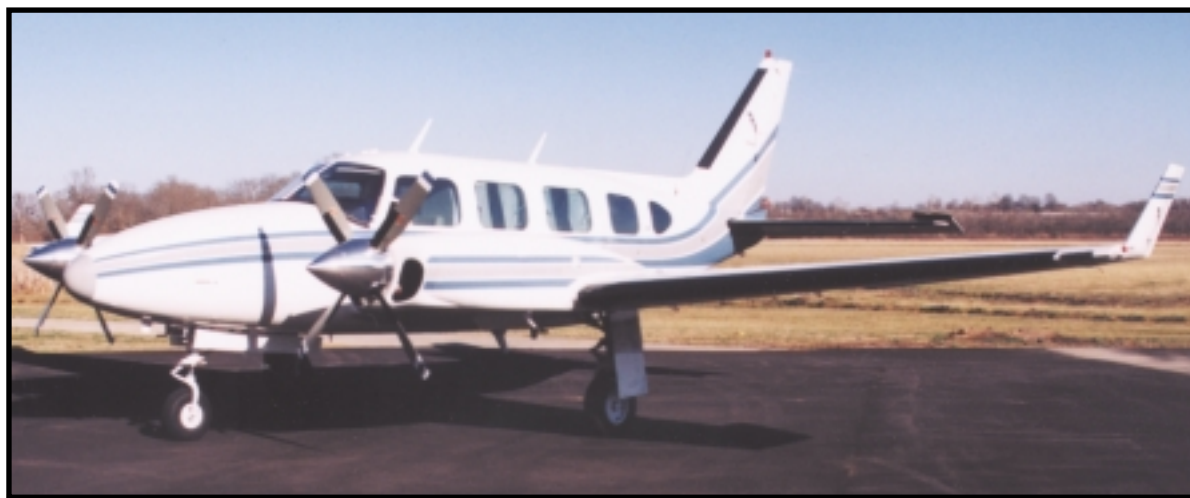
John Baugh says his Navajo performs much better, is much more stable, quieter, and smoother since he had Colemill's Panther conversion performed on it.
